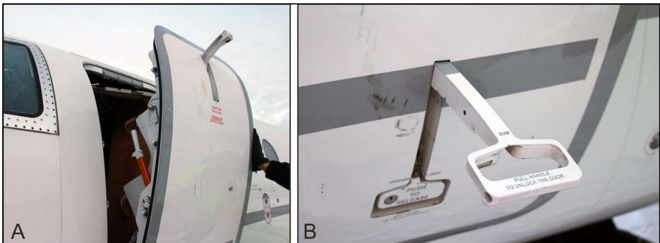
Image 3: 3A: The door in the process of opening, the ground support leg has come out. 3B: A close-up of the stirrup handle. Photo: SIAF
