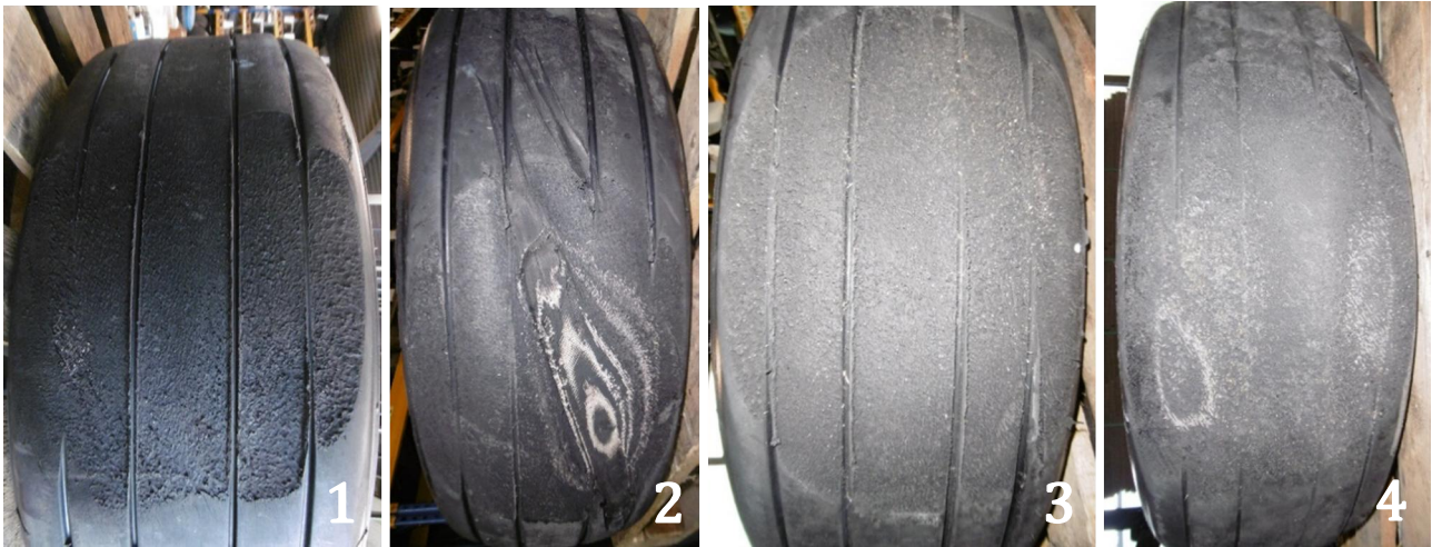
Figure 14. Damage to the mainwheel tires. The tires are arranged to correspond to their position on the airplane as seen from the rear. (Photos: CityJet)
