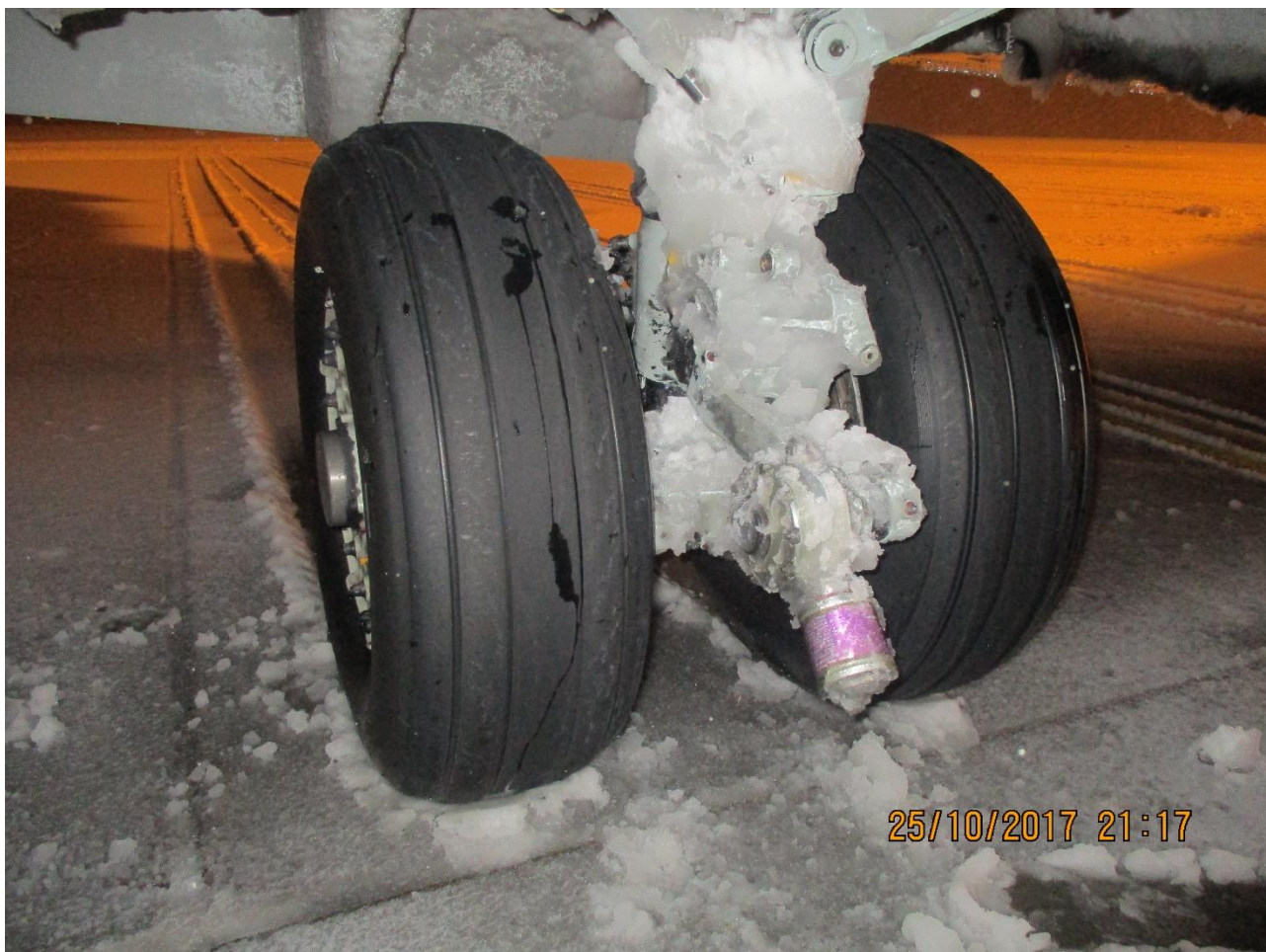
Figure 5. This close-up was taken on the apron approximately 50 min after landing. The airplane taxied into this position and stopped approximately 15 min after landing. No significant amount of fresh snow has fallen on the underwing areas, and by examining the track depth it can be estimated that the slush was over 10 mm deep at the time of the landing. Ground temperature expedited the transformation of snow into slush. (Photo: Police)
