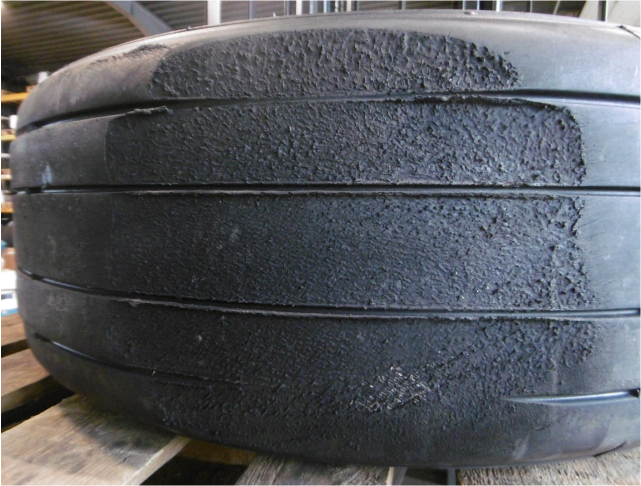
Figure 15. Mainwheel tire #1. Evidence of reverted rubber hydroplaning is apparent on the tread. The tire did not contact the runway edge lights. (Photo: CityJet)
