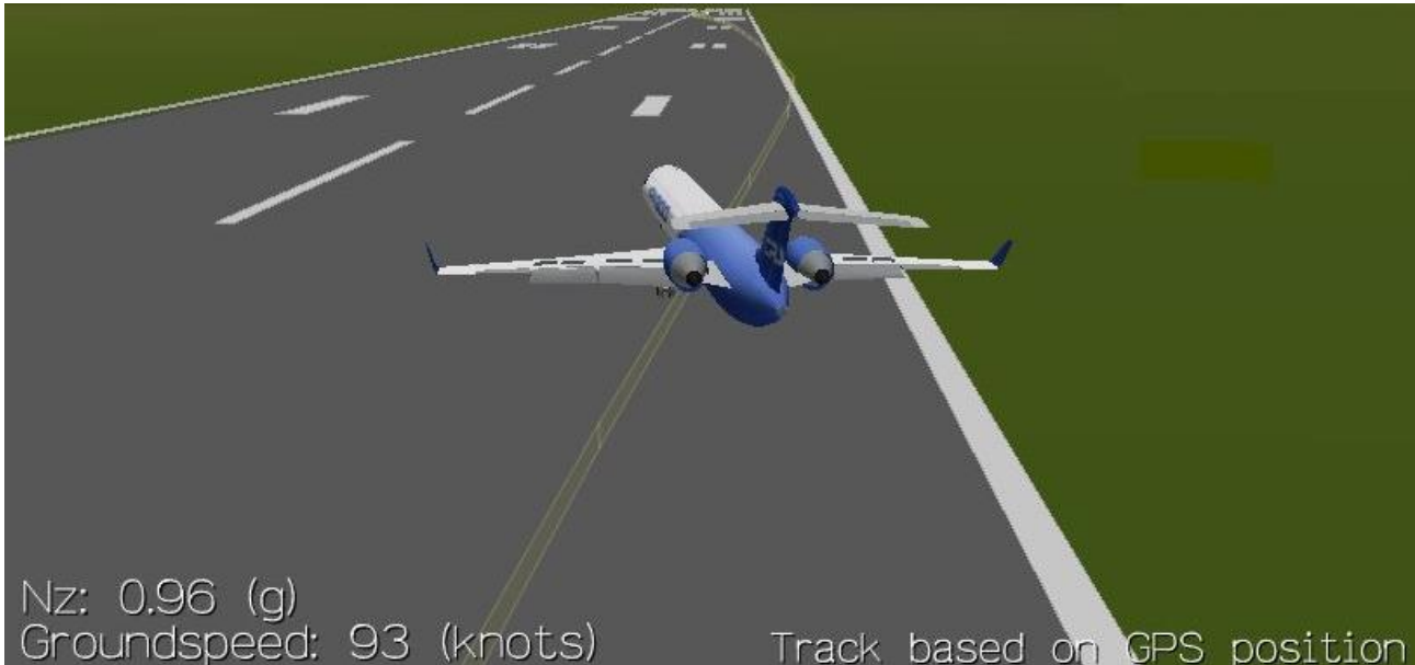
Figure 3. A snapshot from the flight data recorder -derived animation shows the skidding airplane veering off the runway. At this point, groundspeed is approximately 170 km/h, and the airplane tracks as indicated by the yellow line that is based on the locations of GPS points obtained from the recording. The actual paved area extends beyond the white runway edge line, but this is not shown in the picture. The tires did not leave the paved area. (Photo: Insight™ ProView)
