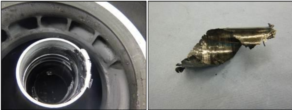
Figure 12. A failed journal bearing and associated damage. (Photos: Hamilton Sundstrand CSC Maastricht BV / UTC Aerospace Systems)
