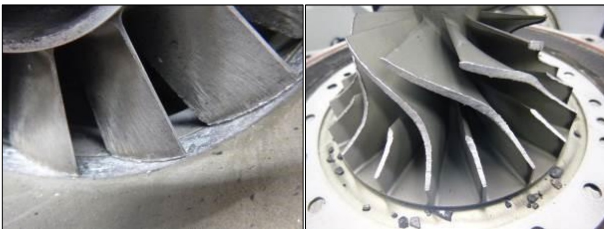
Figure 11. On the left, cooling fan blades showing signs of rubbing. On the right, similarly damaged T2 turbine blades. The T1 turbine exhibited similar damage. (Photos: Hamilton Sundstrand CSC Maastricht BV / UTC Aerospace Systems)
