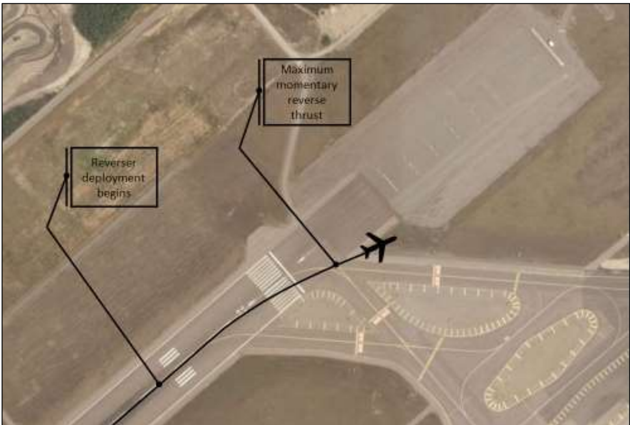
Picture 2. Thrust reverser deployment and final position of aircraft. (Plan view: Orthophoto ©National Land Survey of Finland 4/2018, overlays: SIAF)
