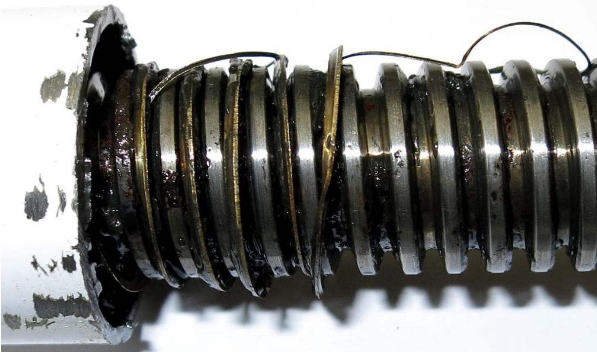
Figure 5. After the grease had been washed away, the bronze threads cut off from the nut assembly were found right at the root of the screw assembly. The nut thread fracture surface was about 0.4 mm wide, which corresponds to the fracture surface that can be seen in Figure 3. (Photo: Safety Investigation Authority, Finland)
