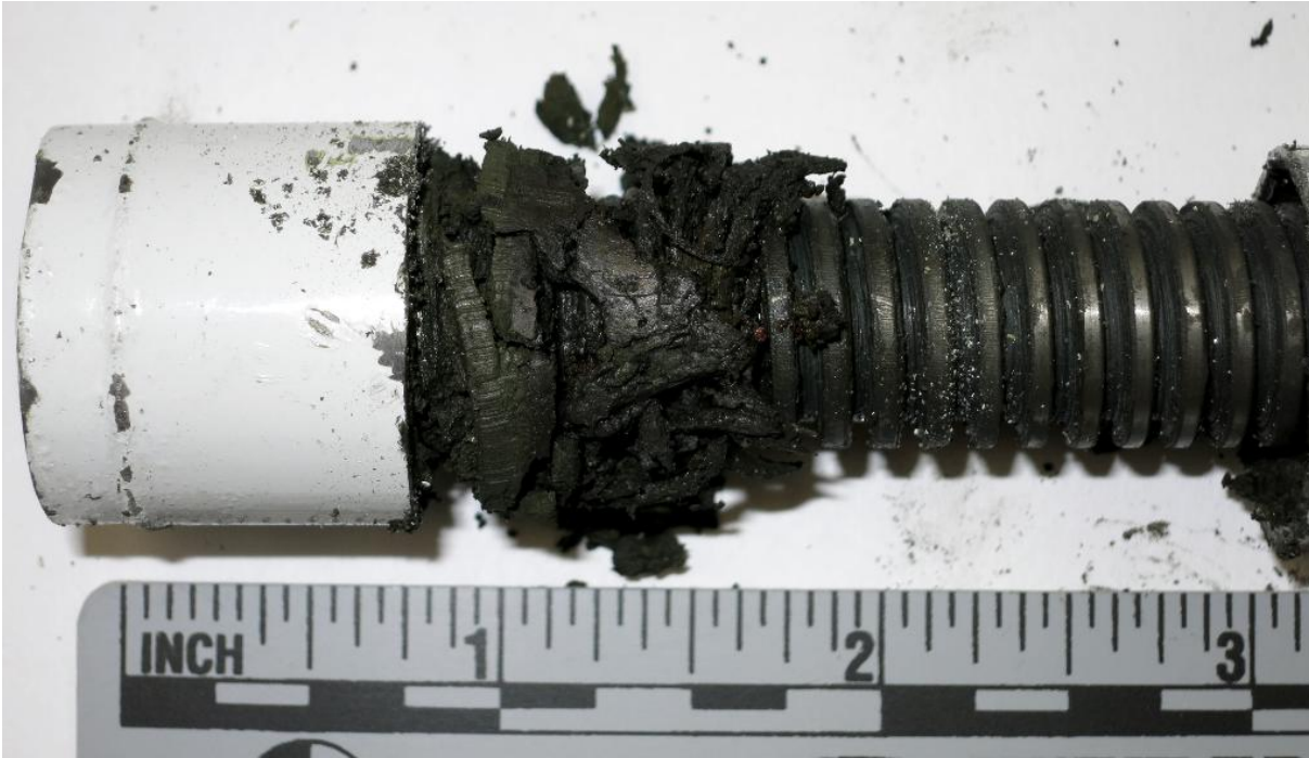
Figure 4. The actuator screw assembly housing was cut open. Lubricating grease and bronze particles had deposited right at the root of the screw. Layers of different colour could be discerned in the grease. A small amount of red grease was found lowest at the bottom. (Photo: Safety Investigation Authority, Finland)
