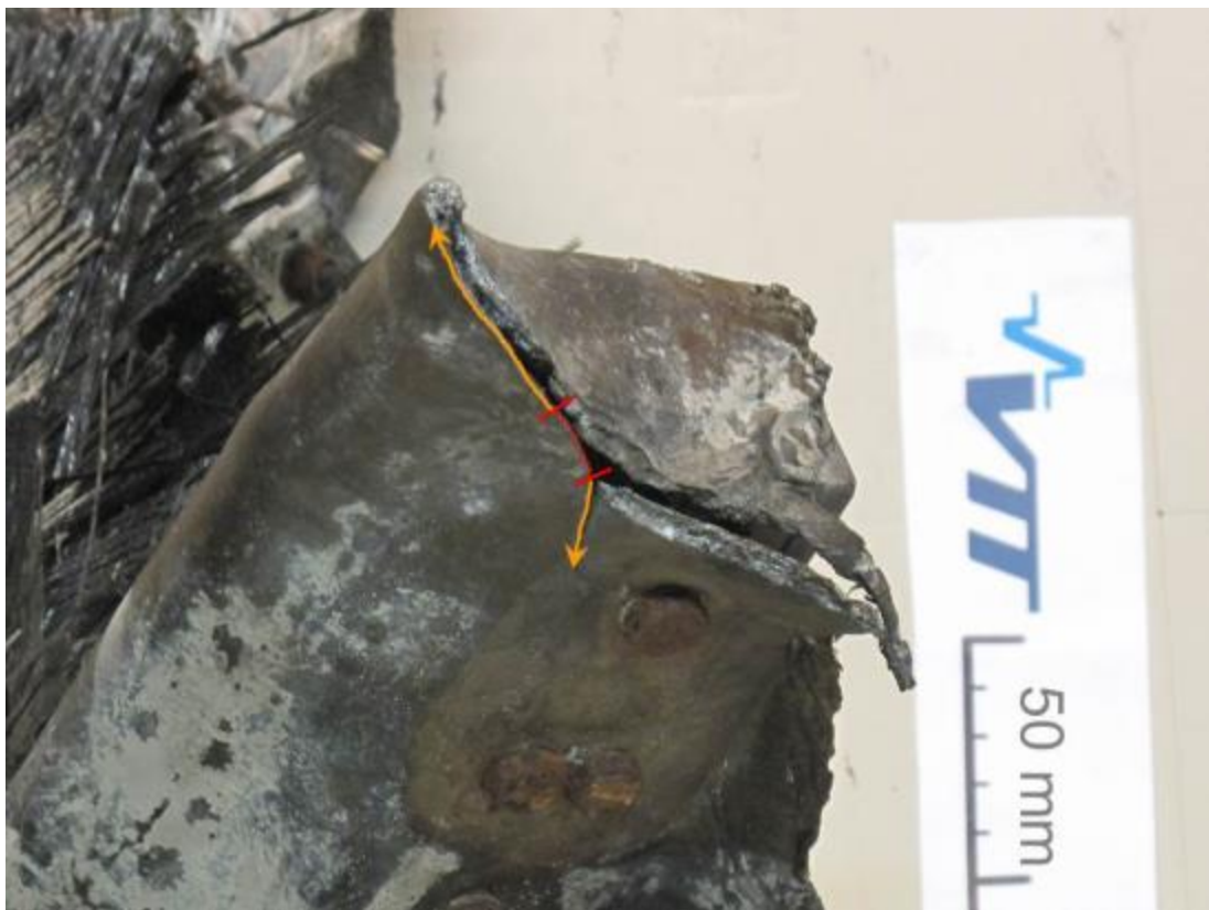
Figure 15. Propagation of the crack in the wing strut (Photo VTT.).
