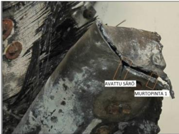
Figure 14. During the material analysis samples were cut from the fracture surface and the crack itself. (Photo: VTT)
