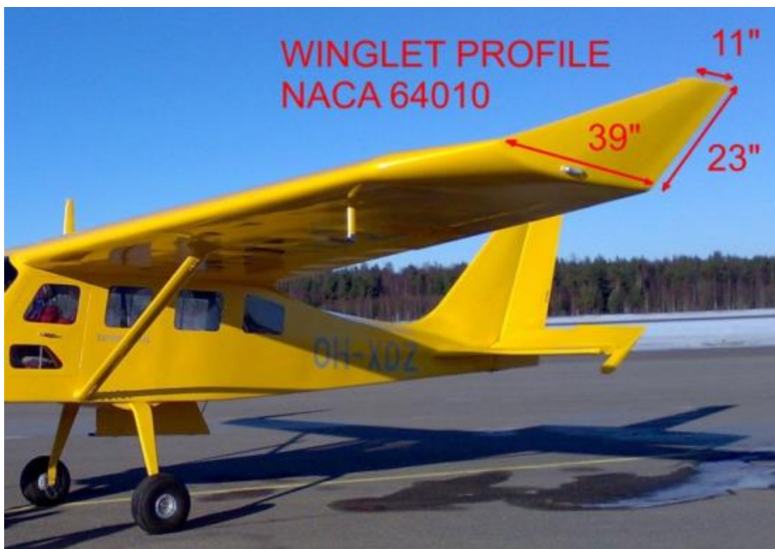
Figure 18. The winglet's main dimensions.
