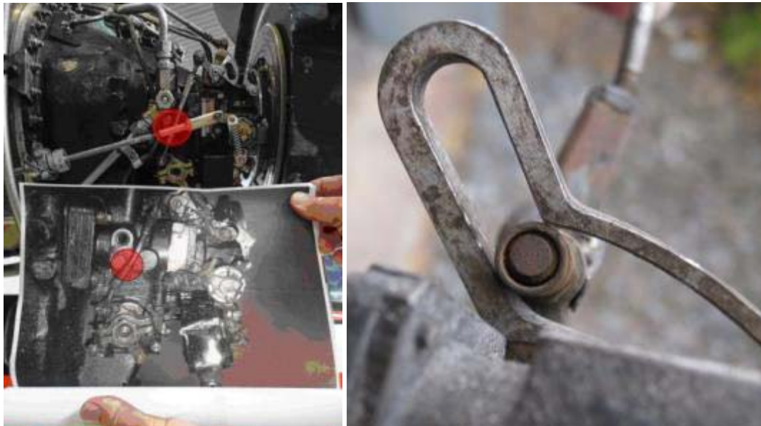
Figure 19. The photo on the left shows governor rod comparisons – a functioning engine above and a photo displaying the OH-XDZ's rod arrangement below. The photo on the right shows the guide which is operated by the engine's fuel control lever.
