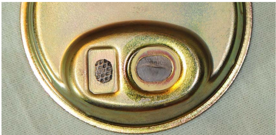
Figure 3. Sideways wear grooves are clearly discernible on the valve cover. Judging by the scoring the cover had constantly been moving between the fully closed and a half open position.
