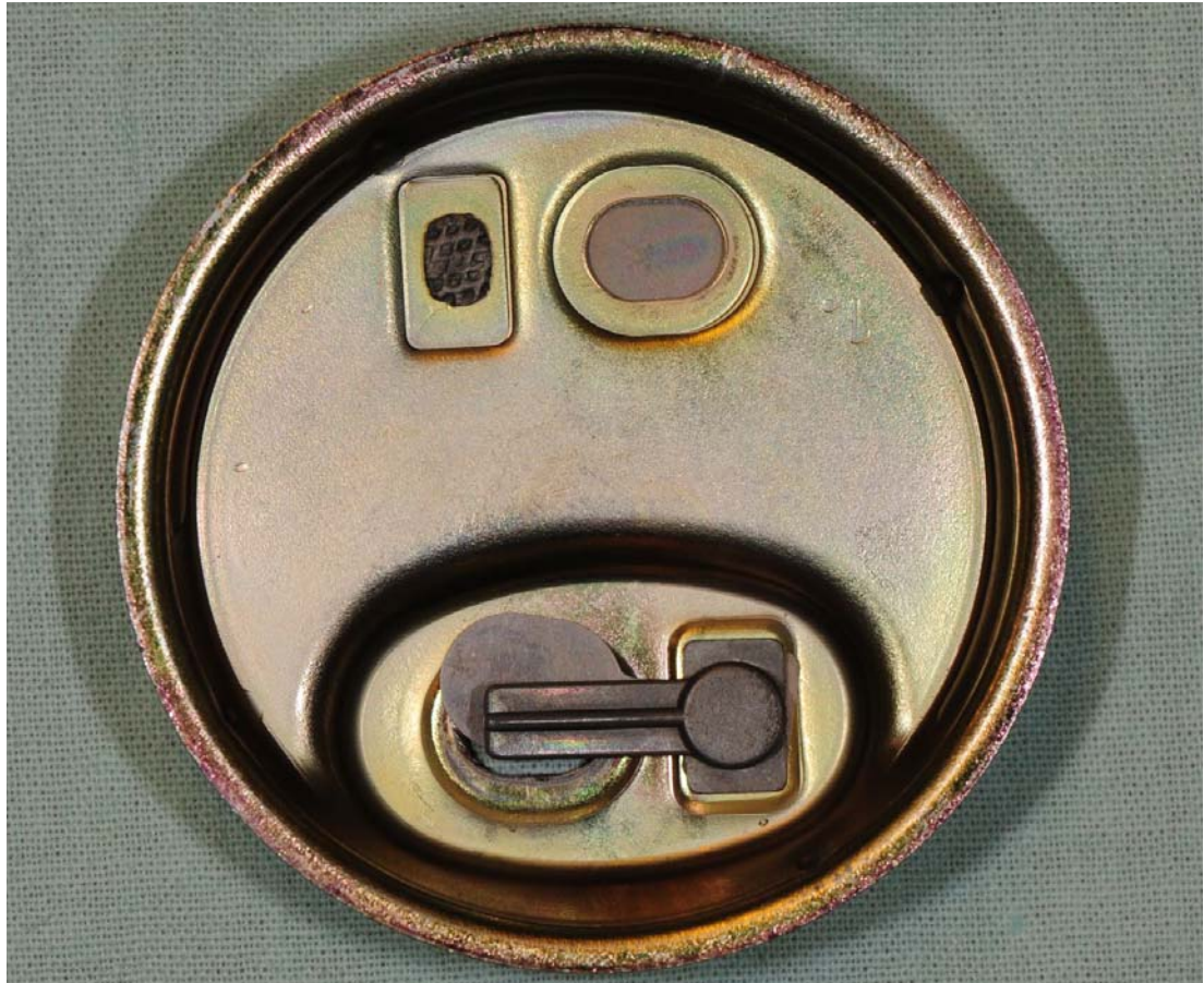
Figure 2. Suction valve cover turned slightly off of its correct position.
