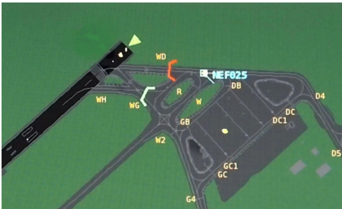
Figure 3. Surface movement radar picture showing illuminated stop bar.
