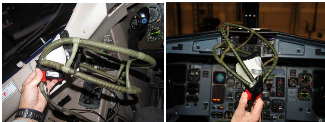
Figure 7. On the left the oxygen mask used in the ATR flight simulator and on the right the oxygen mask used in the aeroplane (OH-ATL). The straps of the oxygen masks used in the simulator had slacked through use.
