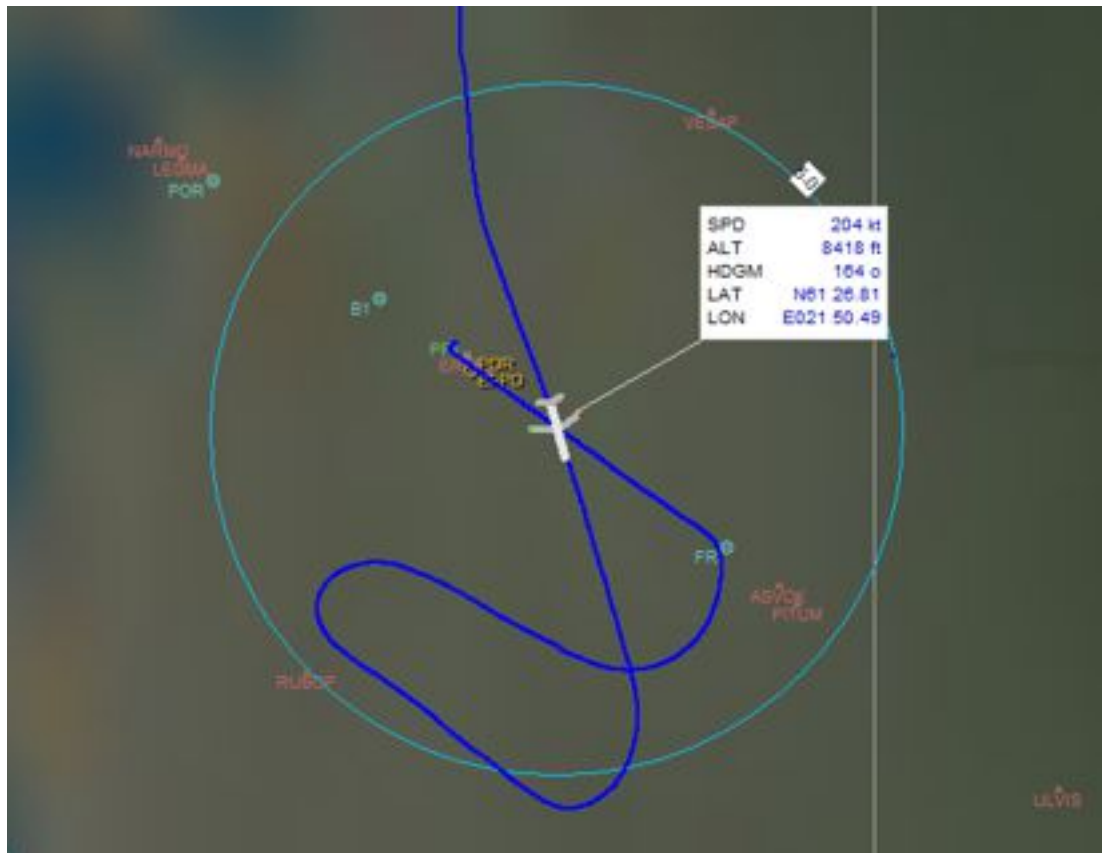
Figure 2. The track of the occurrence flight before the landing (Image: Flybe Finland Plc)
