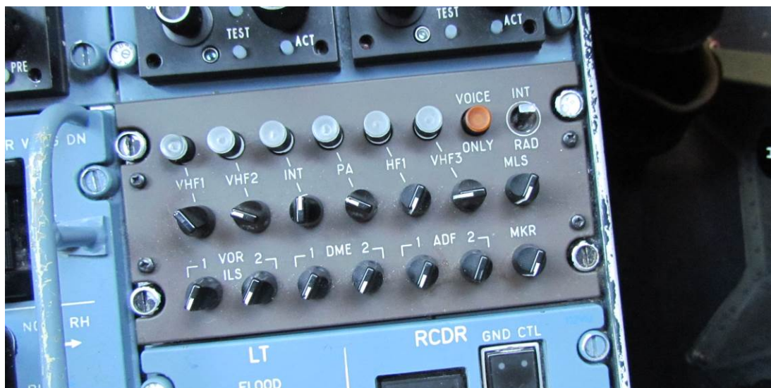
Figure 6. Audio control panel.
