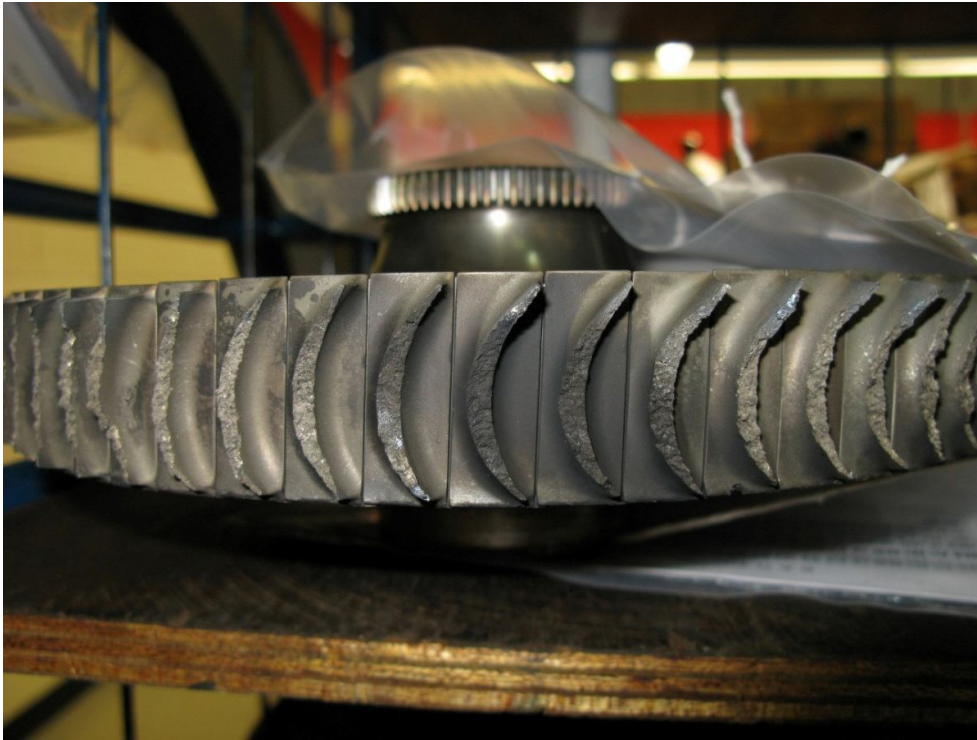
Figure 8. Fracture of all blades caused by overload in the third stage of the turbine.
