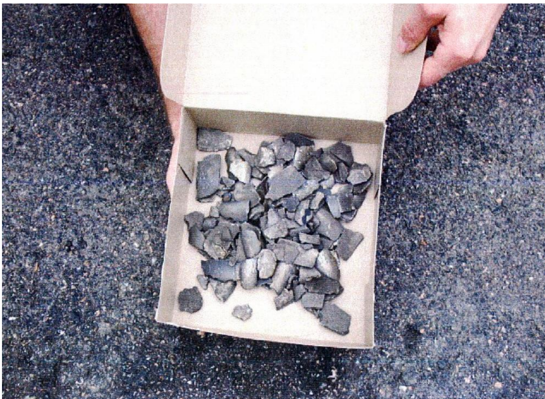
Figure 4. Pieces of engine found by the airport maintenance unit on runway 22R. The runway surface is shown in the background.
