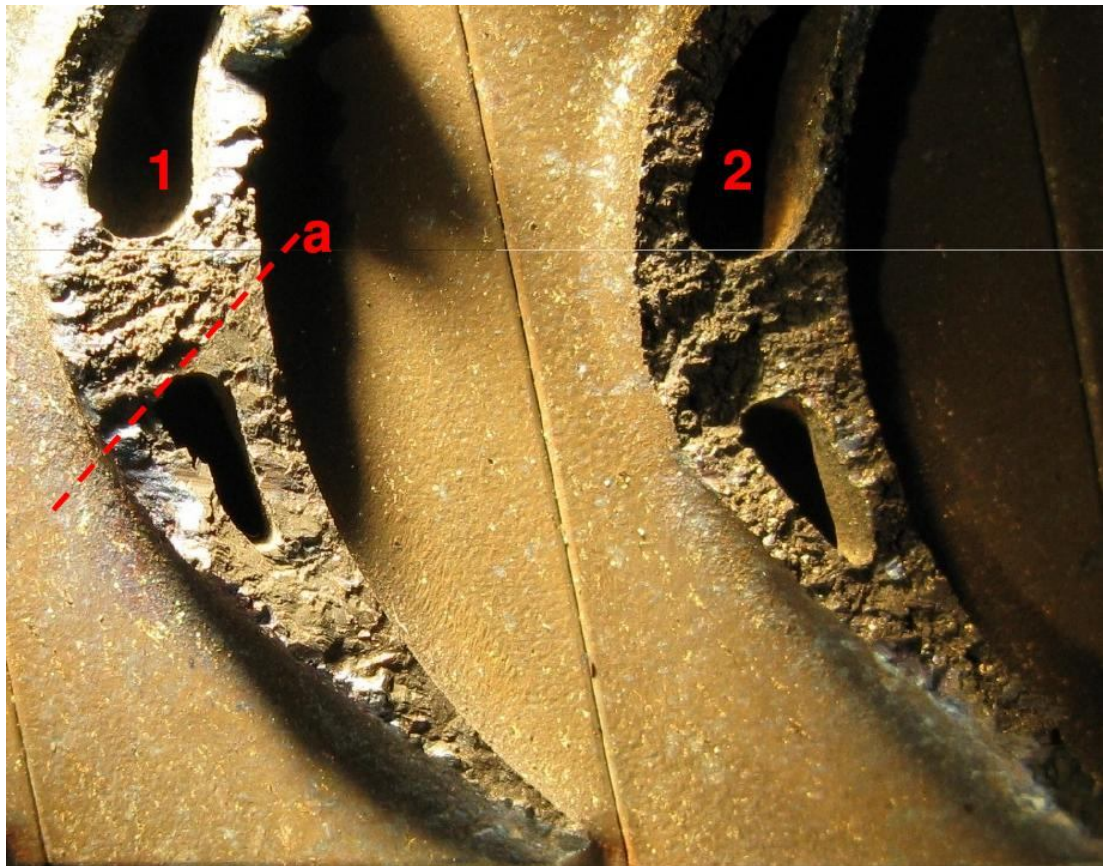
Figure 7. On the left, a turbine blade (1) where the fatigue fracture can be seen as a smoother area up to line (a). Compare with the other blade (2) on the right with an overload fracture surface across the entire root.
