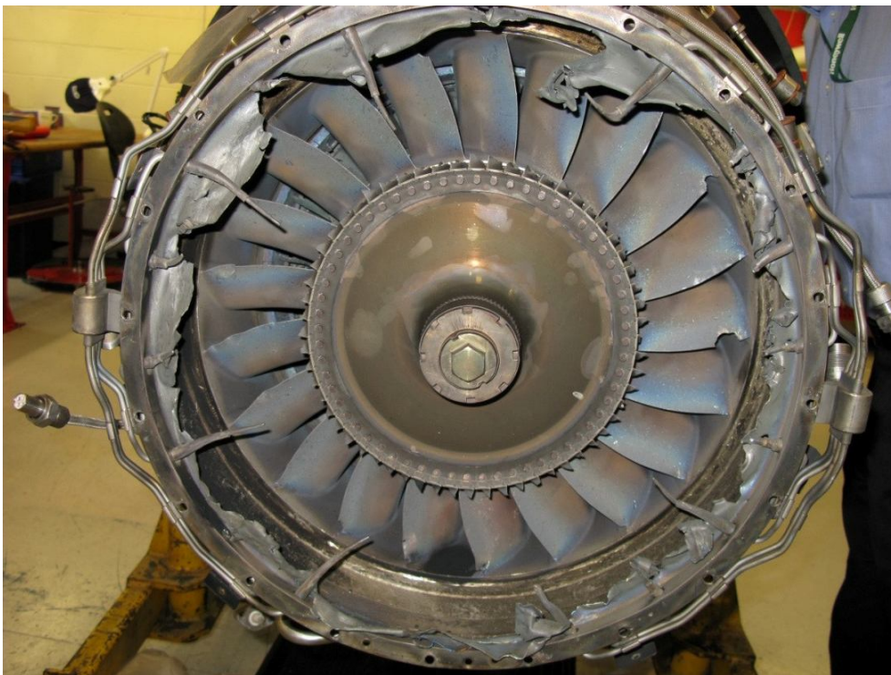
Figure 9. Damage in the fourth stage of the LP turbine was caused by the detachment of the turbine blades. The LPT4 turbine blade shroud was damaged, and the containment flange was melted but complete. The EGT probes were severely distorted.
