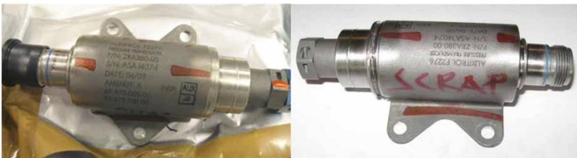
Pressure transducer s/n ASA14074 removed from OH-LTS's left engine.
