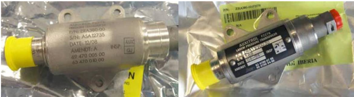
Pressure transducers removed from OH-LTO's left engine; s/n ASA12735 on the left and s/n 188 on the right.
