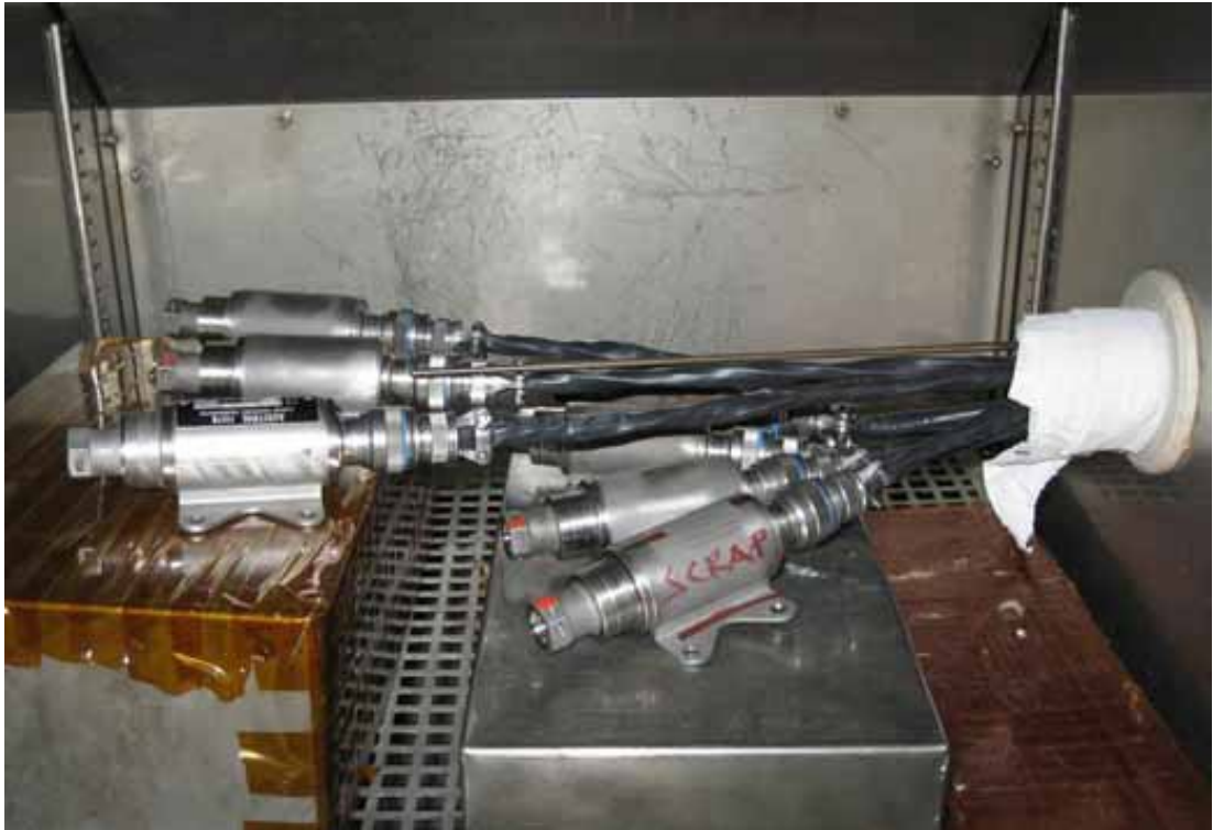
Figure 18. Pressure transducer output signal stability test arrangements in the test chamber. Source: Esterline-Auxitrol 5 .
