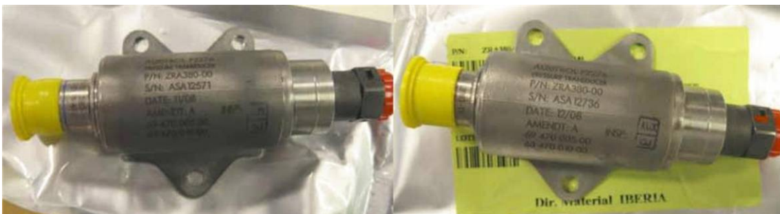
Pressure transducers removed from OH-LTO's right engine; s/n ASA12571 on the left and s/n ASA12736 on the right.
