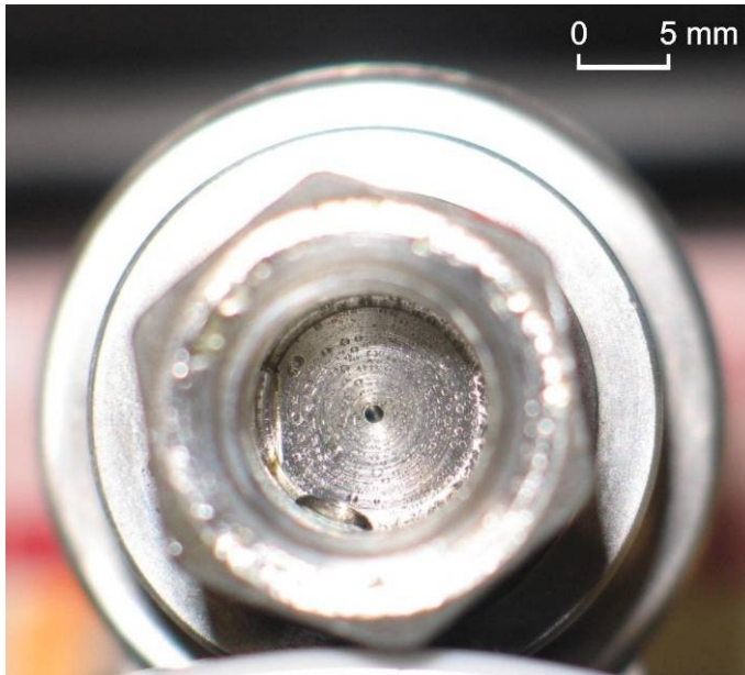
Figure 16. Pressure transducer Pr that was removed from the left engine's bleed air system on 13 Dec 2010. A large drop of water is visible at seven o'clock inside the pressure port. Source: Finnair Technical Services Ltd.
