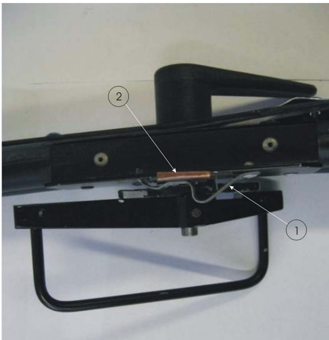
Picture 4. The canopy locking handle, the locking spring holding the handle in the closed position and the additional plate assembled under it. 1. Locking spring, 2. additional plate.
