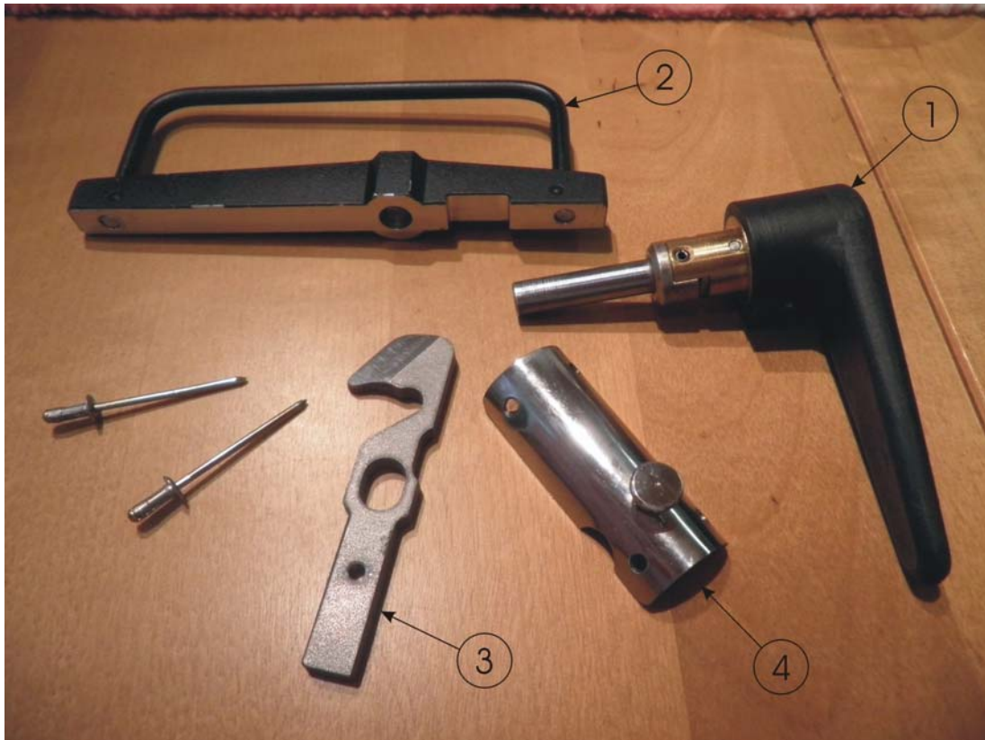
Picture 3. Canopy locking alteration parts delivered for another EV-97 Eurostar aircraft canopy alteration work. 1. outer handle, 2. inner handle, 3. locking hook to be attached to the inner handle, 4. flanged locking pin.
