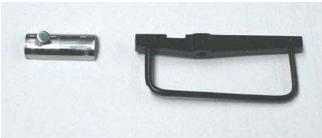
Picture 5. The parts to be changed to the locking mechanism according to bulletin number EV-97-009a.
