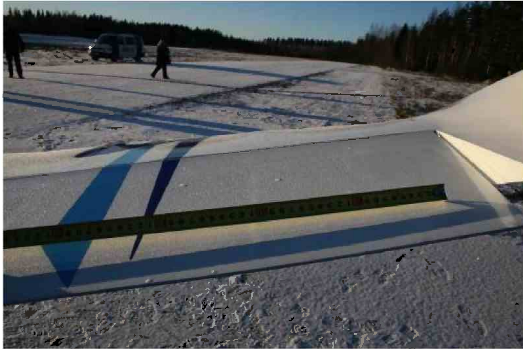
Figure 2. Hoarfrost and frozen water droplets on top of the wing.
