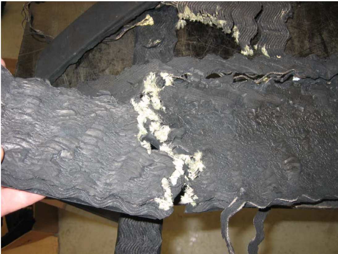
Figure 3. The detached tread and aramid fibre (white material)
