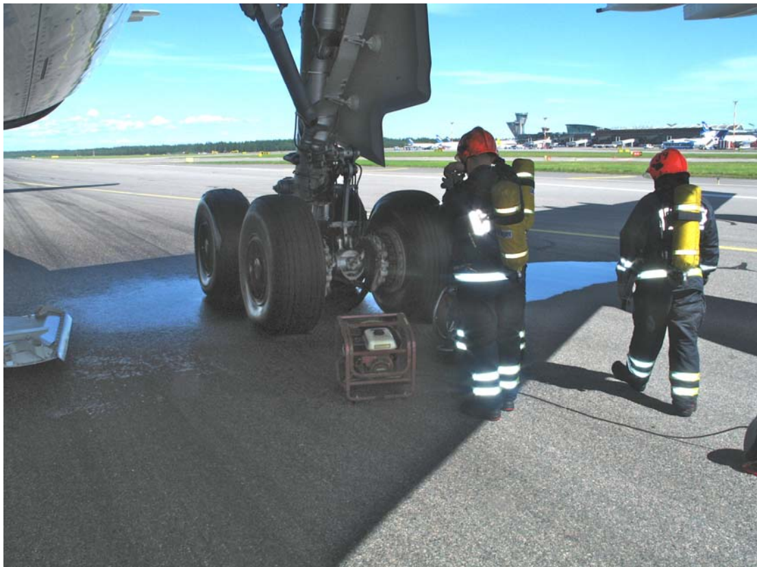
Figure 1. Hydraulic fluid on the runway
