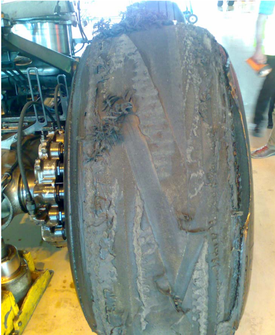
Figure 2. The damaged tyre
