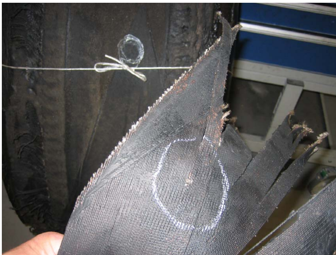
Figure 4 The FOD hole on the tyre as well as on the casing belt ply.
