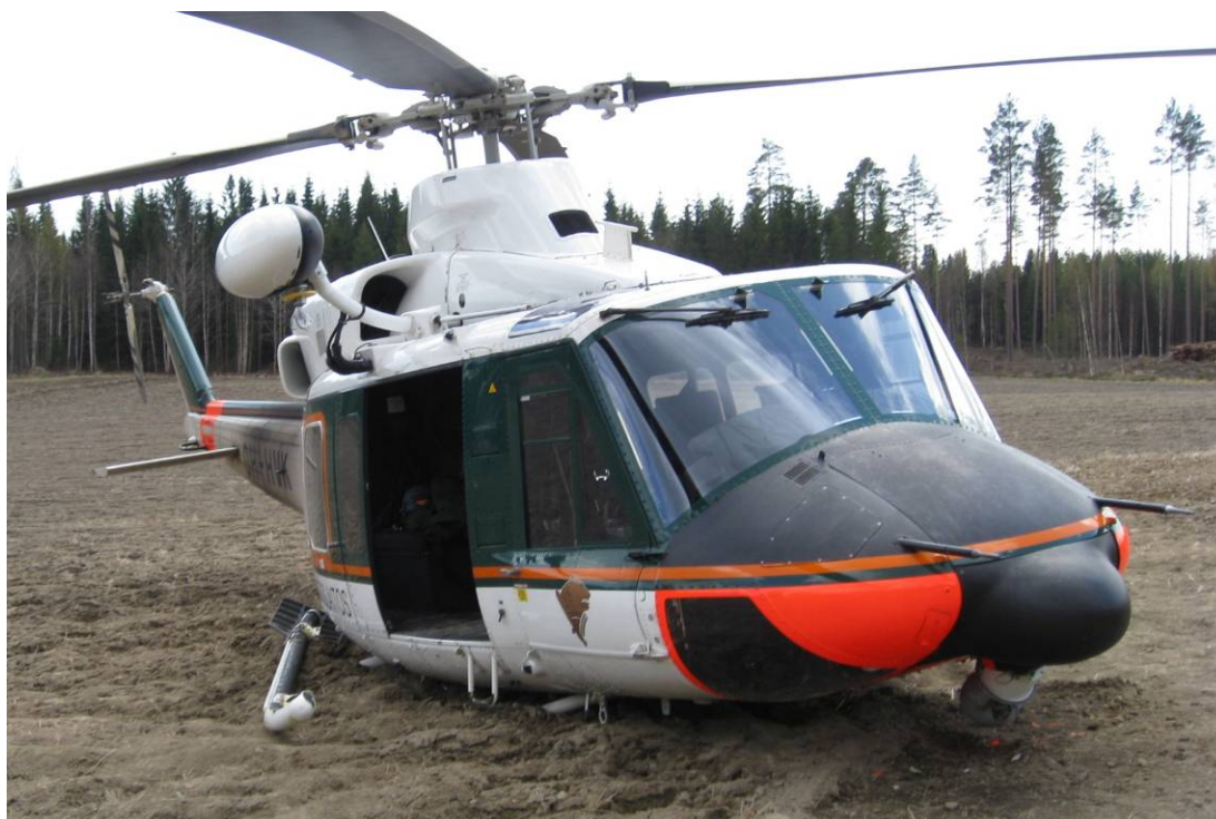
Figure 6. The helicopter on its belly at the accident site.
