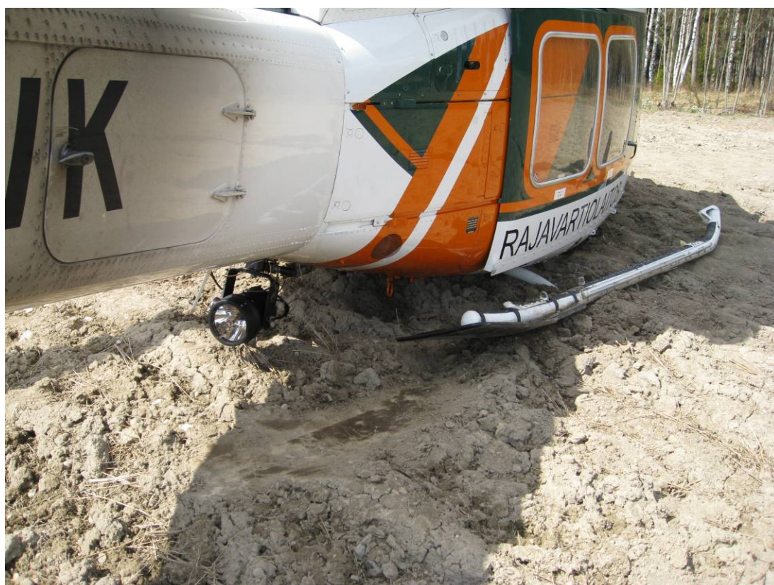
Figure 9. Damage on the right side. The photo shows the skid mark.
