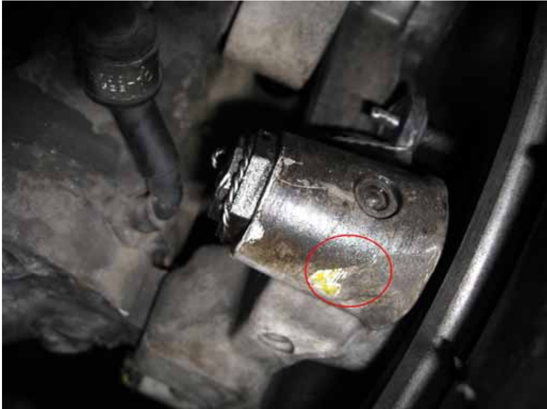
Figure 3. Yellow paint underside of the brake assembly
