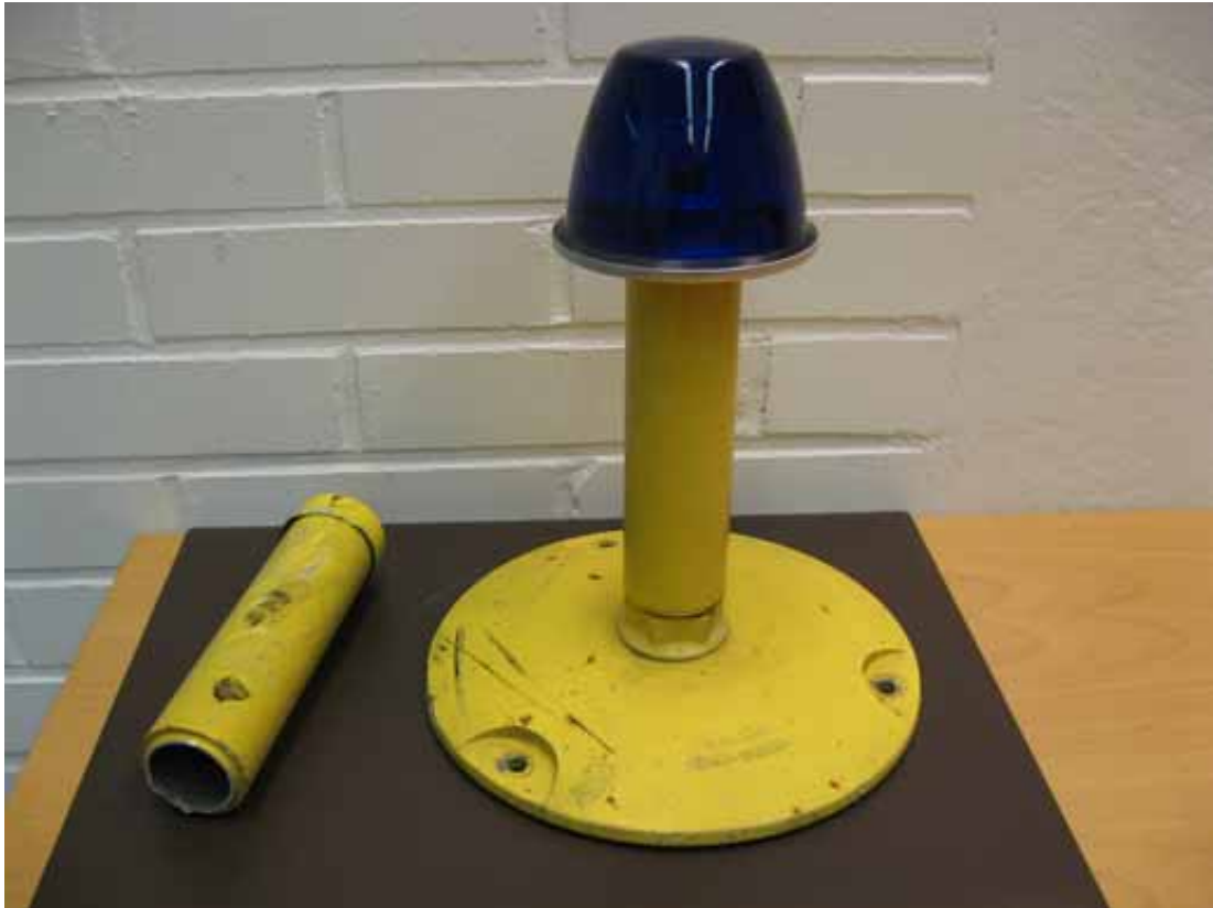
Figure 4. A taxiway lighting fixture and its broken shaft (left)
