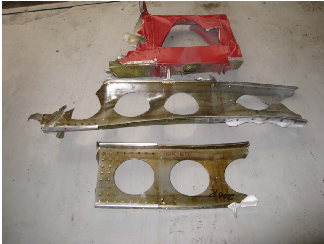
Figure 6. Parts inspected by VTT. Top: part of the stabilator. Middle: part of the left wing spar. Bottom: part of the right wing spar (all of the parts' fracture surfaces were at the left end).
