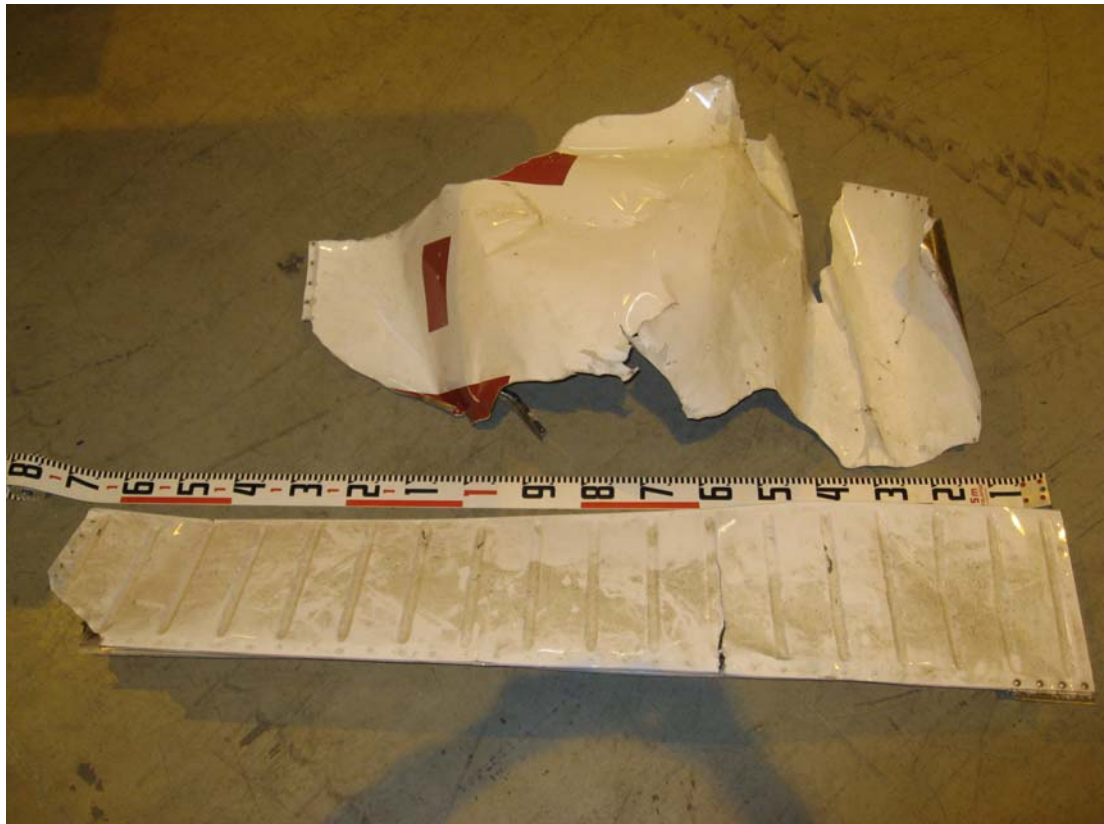
Figure 5. Parts that fell off the aircraft in flight and were discovered in searches.
