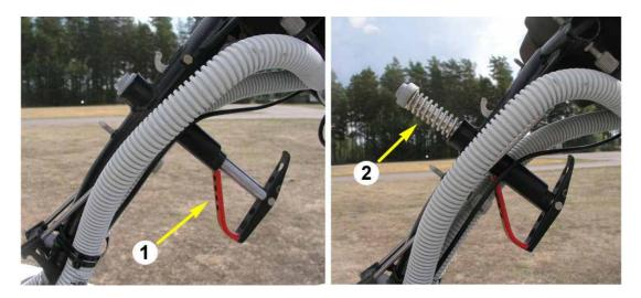
Figure 4. The compression spring locking system of the spring-type canopy jettison mechanism. The left-hand picture shows the red locking handle (1) in the locked position for canopy mounting. The right-hand picture shows the compression spring (2) in the extended, canopy jettison position.
