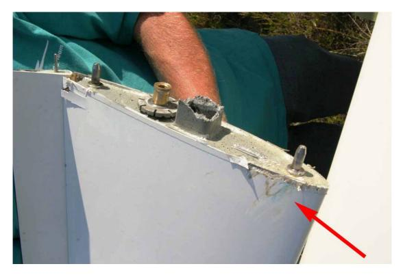
Figure 3. The wing base rib of the separated wing extension of T8. The blue paint trace on the right is indicated by the arrow.
