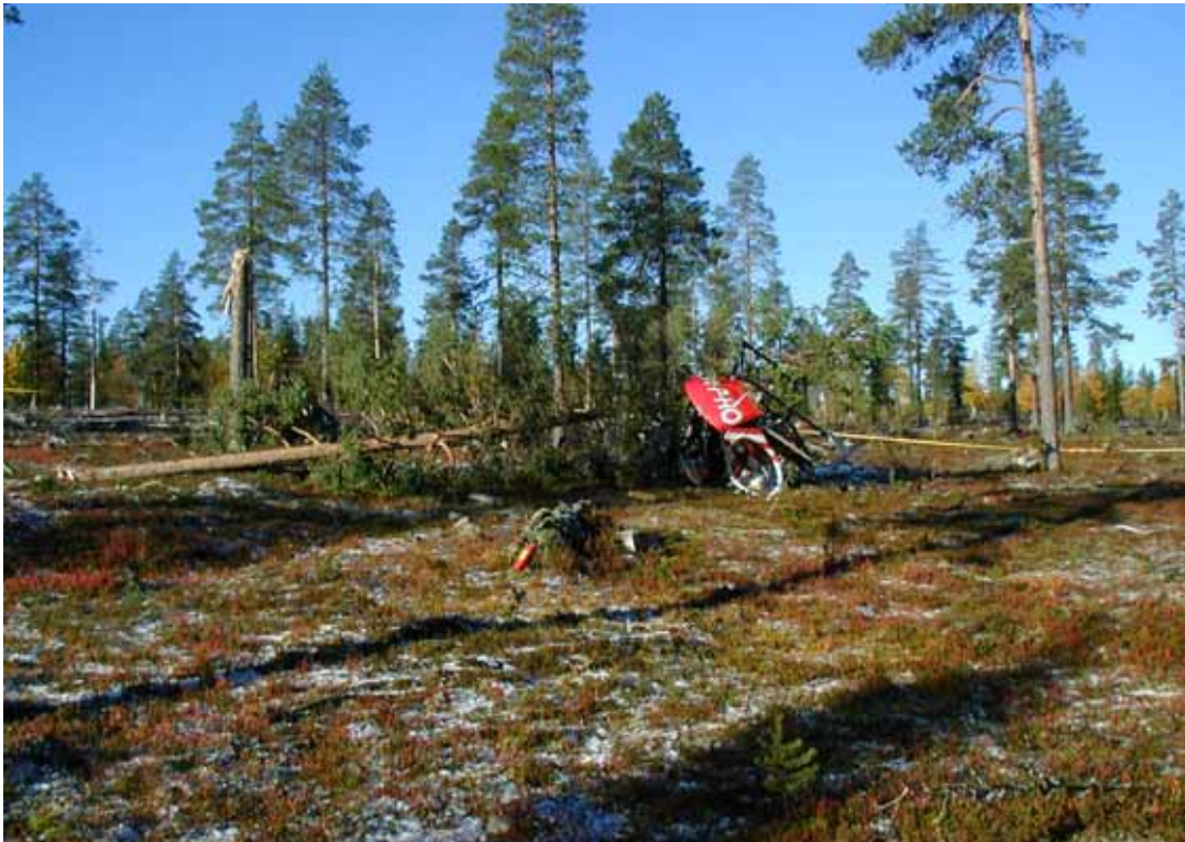
Figure 1. Place of the helicopter impacting on the ground. The helicopter flight direction was from the left to the right. The tree on the left was cut by the main rotor blades.
