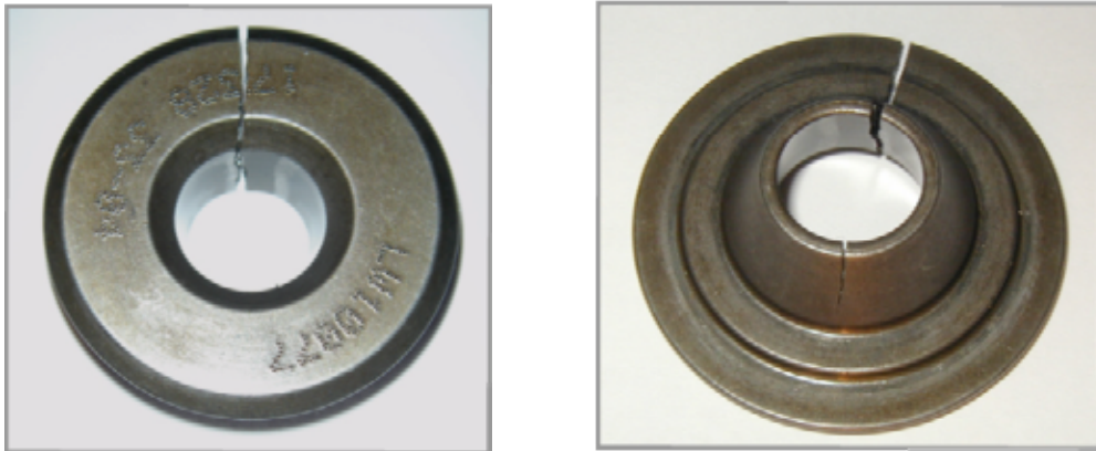
Figure 6. Intake outer valve spring seat of cylinder number 4.
