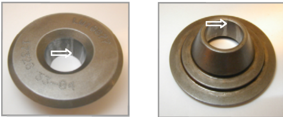
Figure 7. Intake outer valve spring seat of cylinder number 2.
