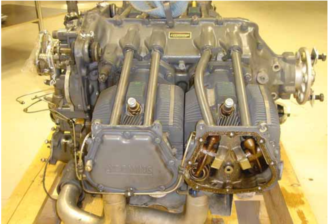
Figure 3. The bent shroud tube of cylinder number 1 intake valve pushrod.
