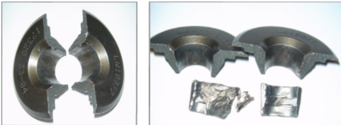
Figure 5. The broken outer valve spring seat and valve retaining keys of cylinder number 1 intake valve.
