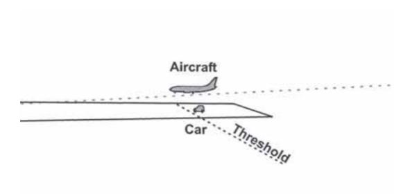
Picture 1. Landing aircraft over the threshold
