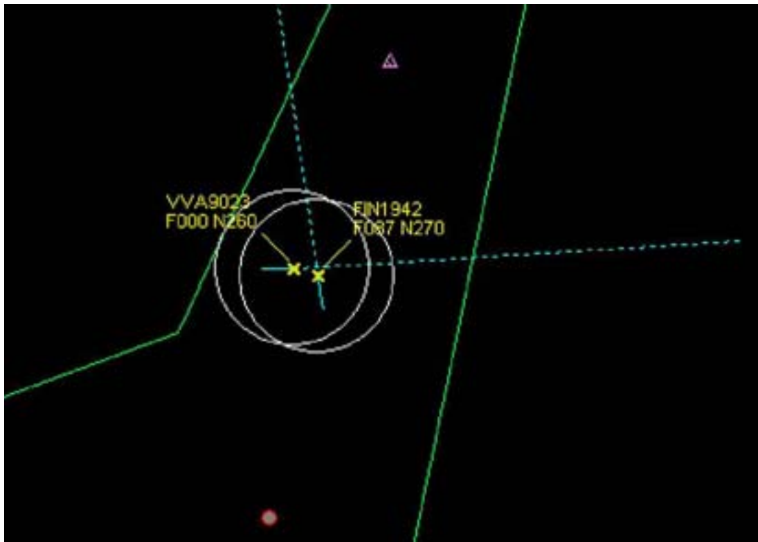
Picture 3. The positions and C-mode altitudes of the aircraft at the passing moment
