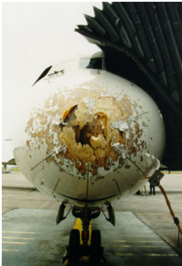
Figure 5. The damaged radome
