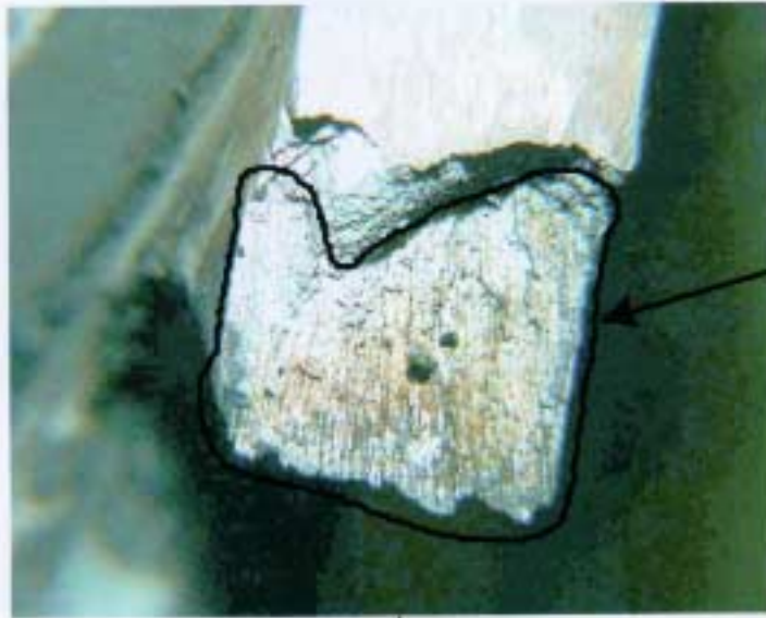
Fracture surface 1a. 50% of the fracture is caused by stress corrosion.
