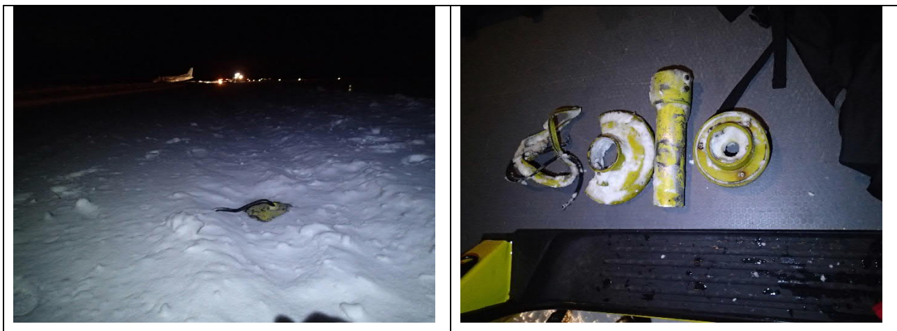
Figure 4. The broken runway edge light. (Photos: SIAF)
