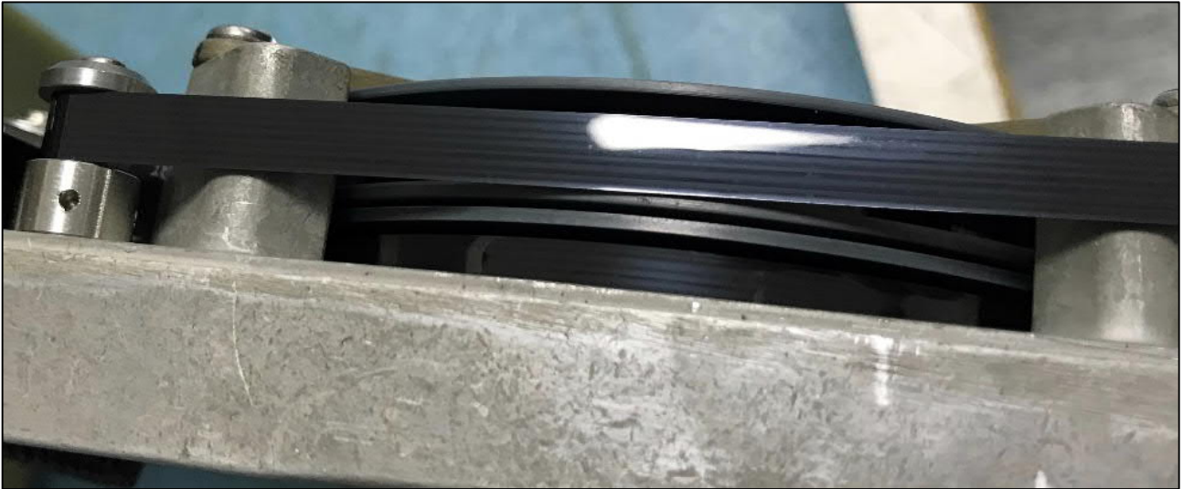
Figure 7 The longitudinal stripes visible in the photo are telltale signs of wear. Tapes that are in good condition do not show stripes. (Photo: AAIB)
